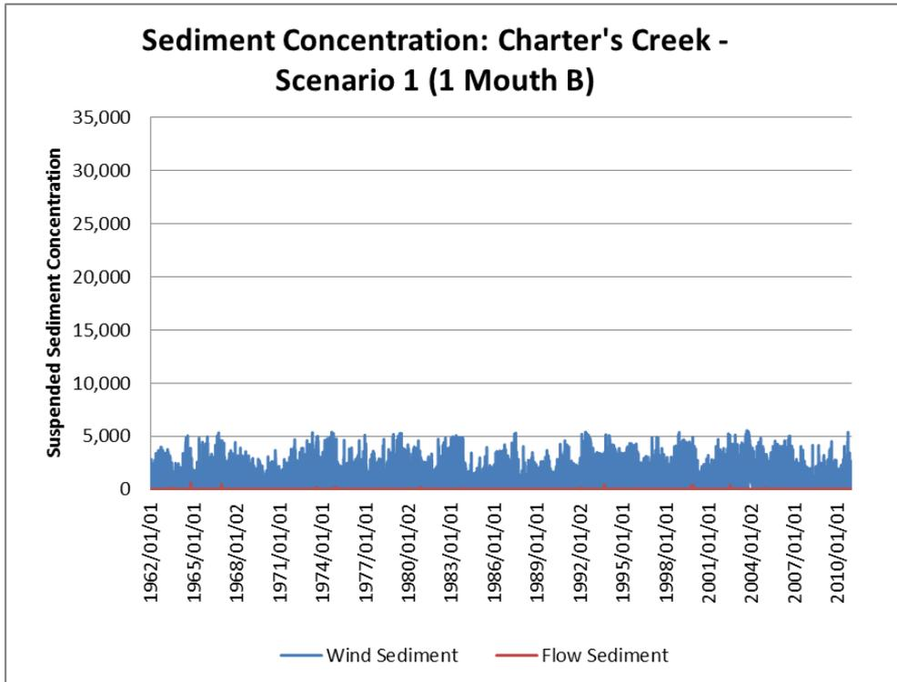
**Figure G-26** Suspended sediment concentration time series (daily data) at Charters Creek: Baseline B
