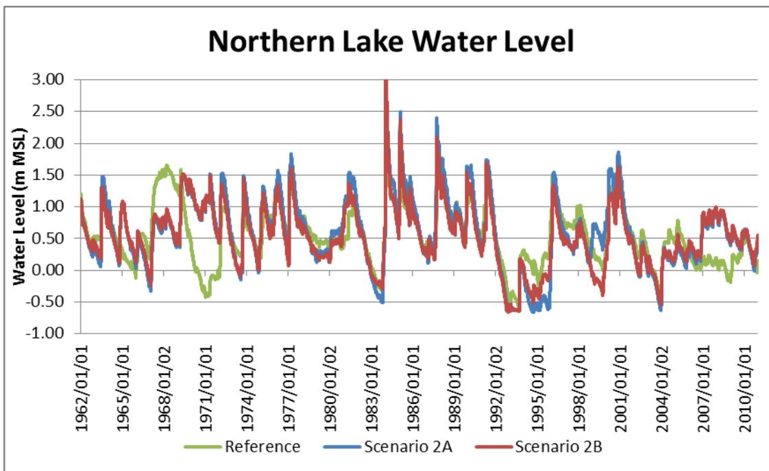
Figure E-15 Northern Lake Water Level (Scenario 2: One Mouth – A and B)
