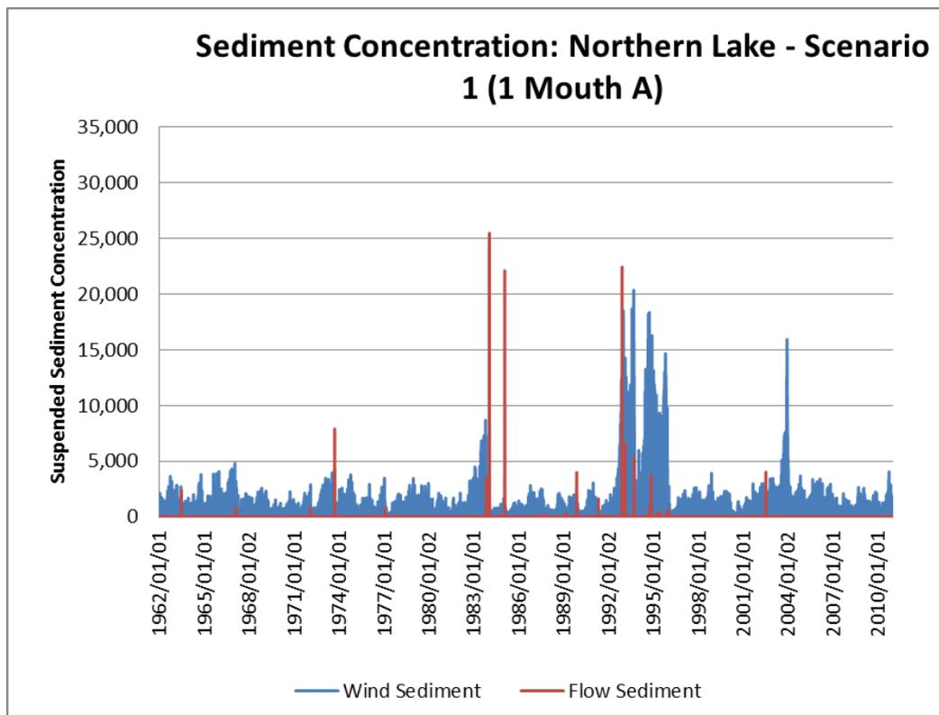
**Figure G-13** Suspended sediment concentration time series (daily data) at Northern Lake: Baseline A
