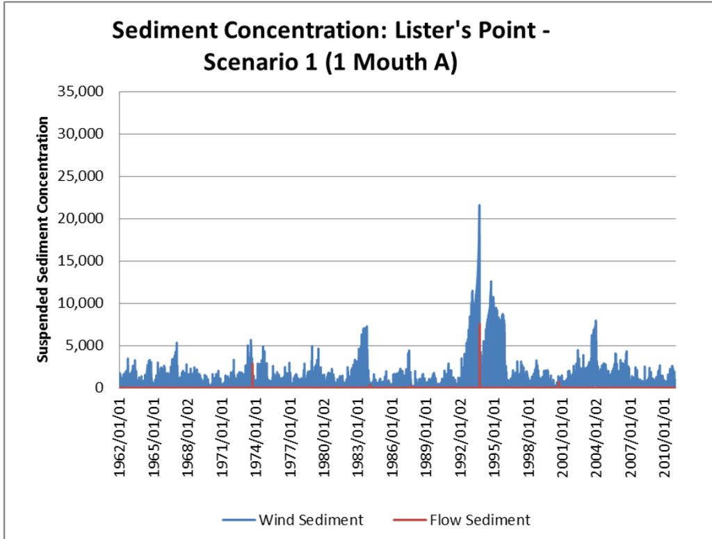
**Figure G-1** Suspended sediment concentration time series (daily data) at Lister's Point: Baseline A
