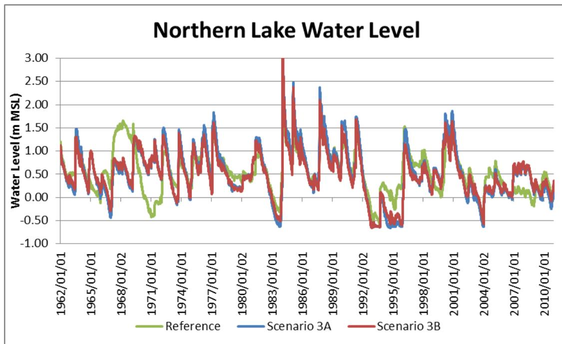
Figure E-21 Northern Lake Water Level (Scenario 3: One Mouth – A and B)
