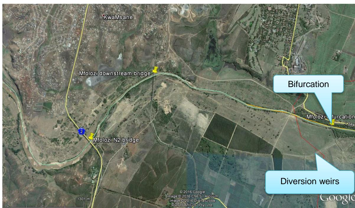
**Figure A-1** Location of the bifurcation and diversion weirs on the uMfolozi River where a new flow gaging station should be established by DWS
