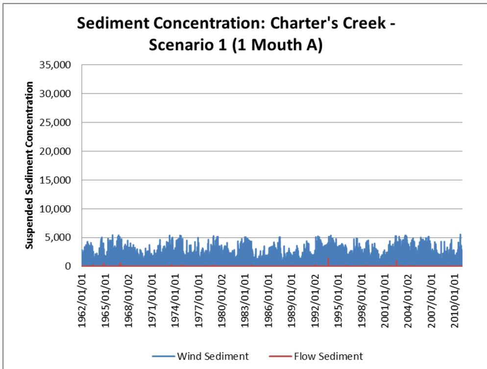
**Figure G-25** Suspended sediment concentration time series (daily data) at Charters Creek: Baseline A
