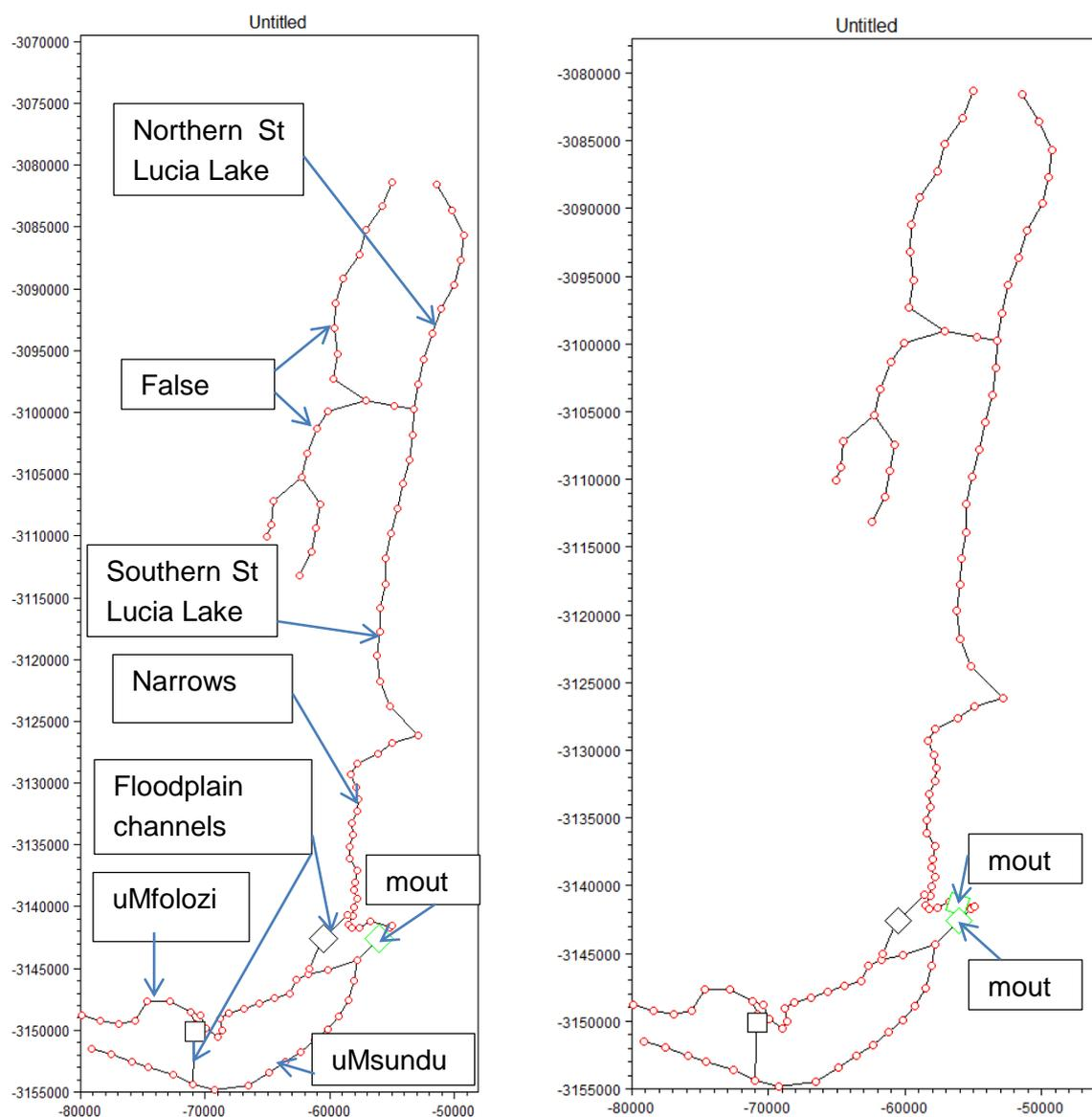
**Figure 4.2.1-2 1D model network layout with single mouth (left) and two mouth setups (right) (iSimangaliso, 2015)**
